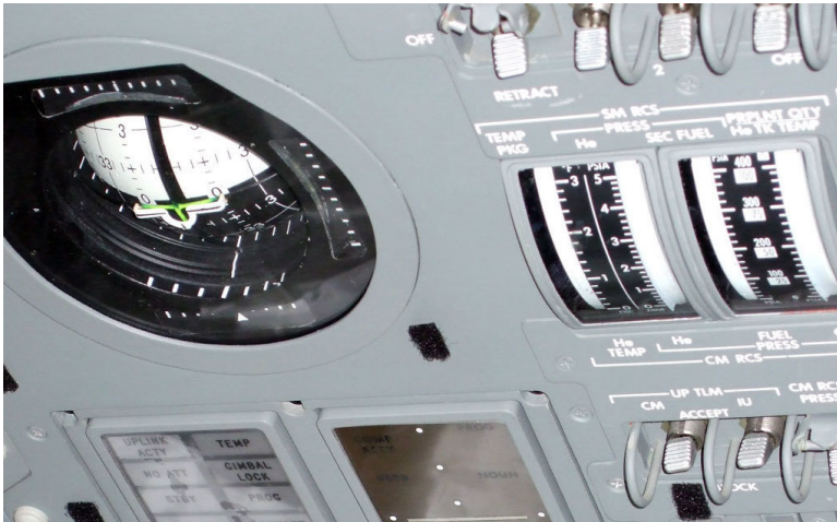
The Flight Director Attitude Indicator (FDAI) of the Apollo Guidance Computer (AGC). Wikimedia Commons.
